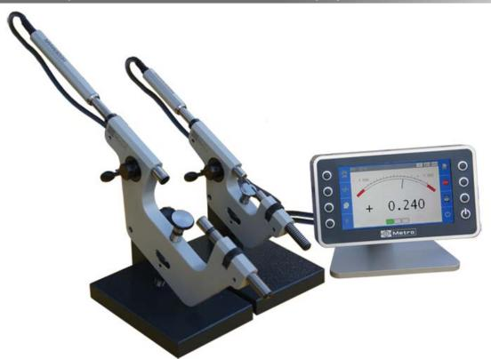
The Metro M2 display unit is particularly adapted to be used with snap gages. The picture below shows an example of application with 2 heidenhain probes mounted on snap gages. The measurement is clearly shown on the M2 screen and the result also with useful green/red indicators.
