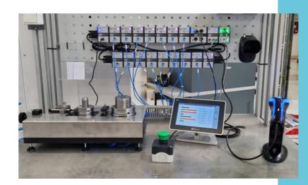
This control system is used to check several dimensions on connecting rods using air gaget. Several parameters are checked, including internal diameters, bend and twist. The measurements are temperature-compensated.
